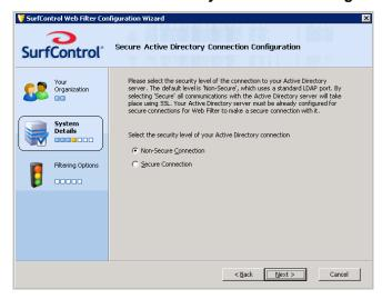
By default a non-secure connection is made to your Active Directory server. To change this to a secure SSL connection, select **Secure Connection**.
